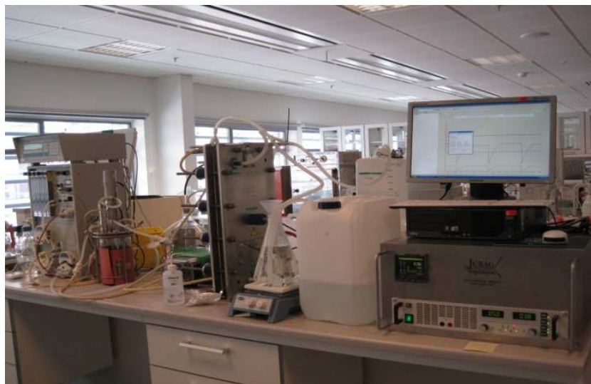
Figure 7: The bench-scale fermentation and separation system consisting of the fermenter and control unit (left), the separation unit (middle), and the separation control unit (right).
