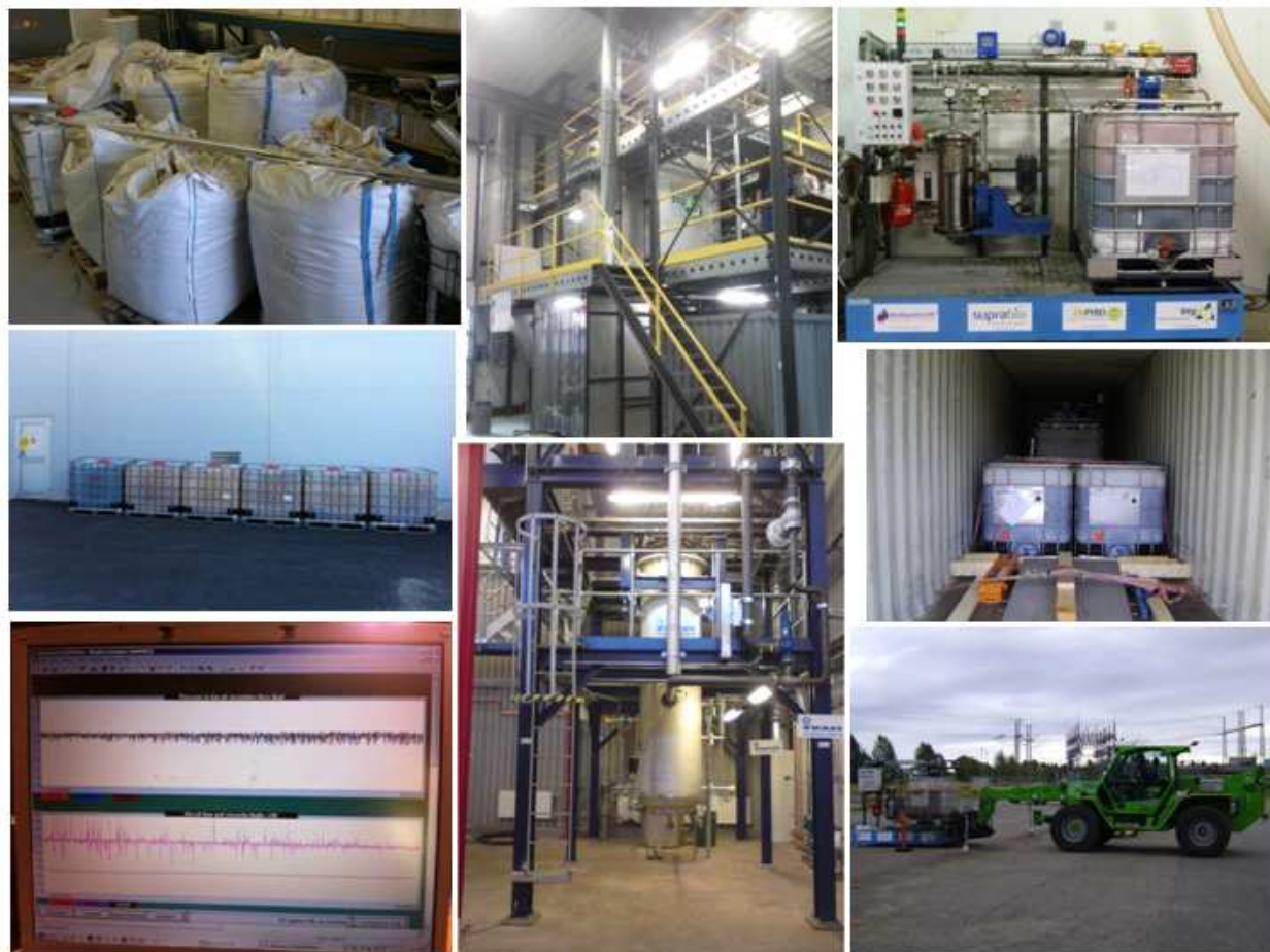
Figure 2: Several photographs of the entrained flow gasification of pyrolysis oil campaigns. Clockwise from left top: Biomass feedstock in big bags. Pyrolysis plant at BTG. Pump skid dedicated to feed the gasifier. Pyrolysis oil and pump skid ready to be shipped. Unloading pump skid at ETC. Entrained flow gasifier at ETC. Stable operation in the gasifier (timeline > 8 hour). Empty IBC's after 50 hour gasification campaign.
